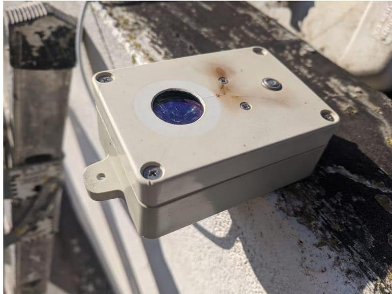
Figure 1. TESS-W stars273 in Malta showing a significant crack on the box top and loss of the window.
